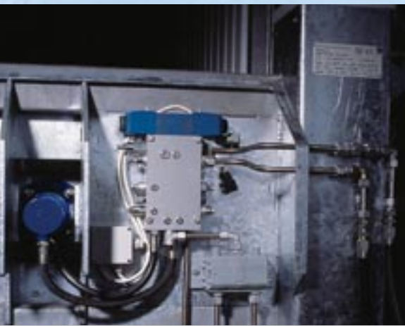
DSI Hydraulic ALU block with secures easy access and service
